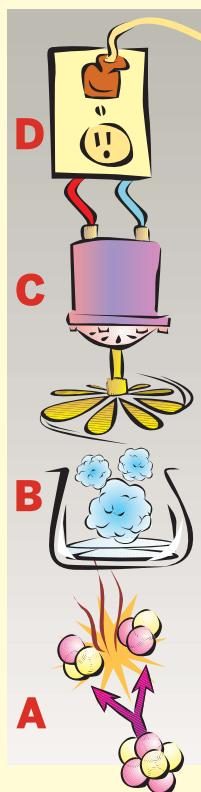
Power plants create electricity by running steam turbines, which are powered either by fossil fuels – coal, oil, natural gas – or by nuclear power. Nuclear technology produces energy by splitting uranium atoms in a process called fission. (A) Fission generates heat that (B) boils water for the steam that runs the (C) turbines, which produce the (D) electricity that we all use – making, for instance, (E) toast for breakfast.
